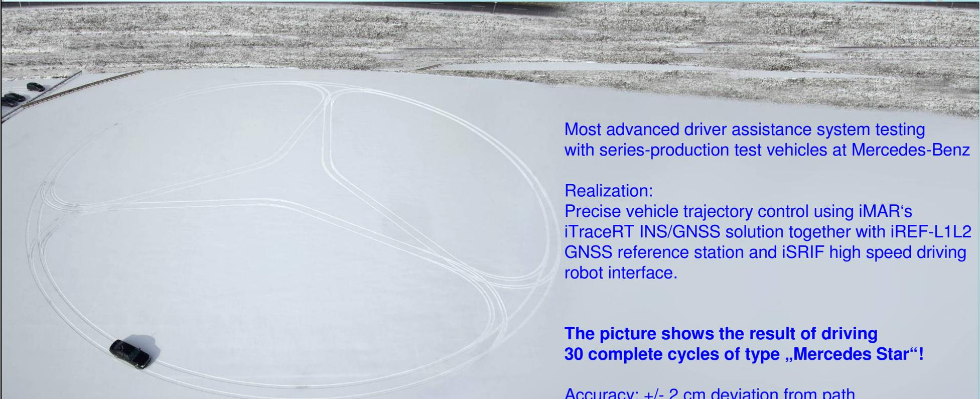
Most advanced driver assistance system testing with series-production test vehicles at Mercedes-Benz
