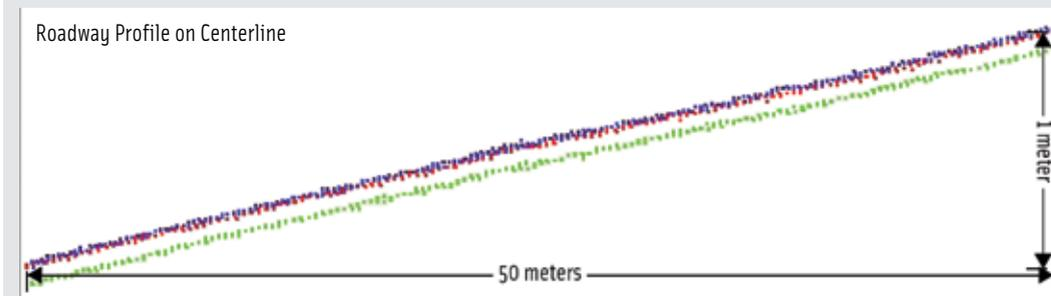
FIGURE 3 Observed vertical bias between three separate passes (red, green, blue) of TITAN on roadway, 10x vertical exaggeration
