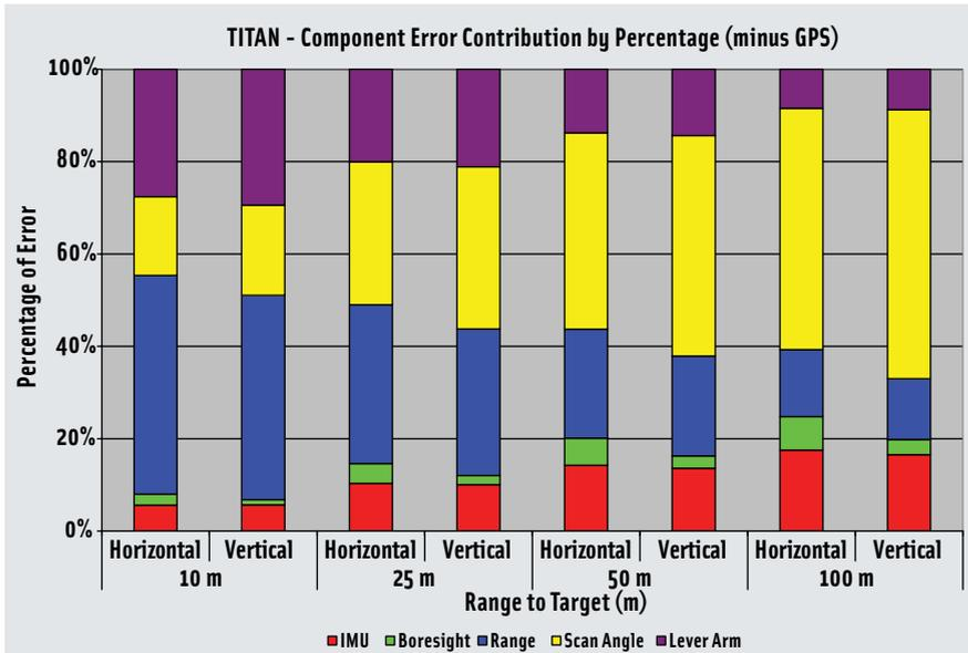
FIGURE 5 TITAN Component Error Contribution by Percentage of Total (from paper by C. Glennie cited in Additional Resources)
