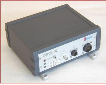
initialisation or fine calibration by the user is required. As an option it is also possible to store all the data of inertial sensors like gyroscopes and accelerometers, odometer and mobile GPS on an internal 4 GByte flashdrive.
