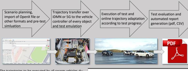
The trajectories to be executed by all swarm vehicles during the Traffic Scenario (up to 10++ VUT, TSVs, SCTs, VEs operable simultaneously on demand) and the timing of the active infrastructure elements ISE (when to change traffic lights, speed limit information etc.) are generated by the iARGUS-CC Control Center software <u>iARGUS-CMD</u> or are
