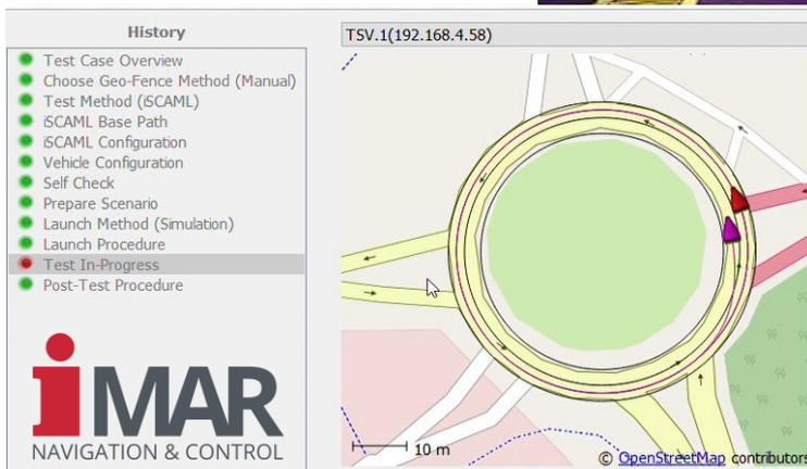
**iMAR's iARGUS-CMD Control Center Software and IPG's CarMaker now have common interface to provide a holistic toolchain for automated driving tests**
