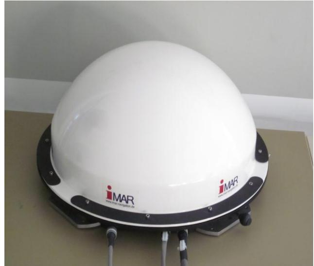
The system is designed for high angular rate and high angular acceleration ( $> 300 \text{ }^\circ/\text{s}^2$  ;  $\pm 300 \text{ }^\circ/\text{s}$ ) at high bandwidth. It can be operated on speed boats as well as on standard warships in heavy seas or on trucks in off-road condition. It supports tracking of stationary or moved targets. Furthermore systems for stabilization of optical devices like IR cameras, laser designators and Laser Range Finders for aircraft or UAVs are available.
