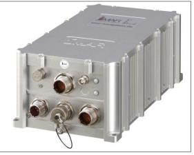
Kalman filter for data fusion incl. gyro compassing, free inertial or dead-reckoning navigation etc. The iNAT-RQH-400x family is available in several performance classes, down to 0.001 deg/sqrt(hr) angular random walk.
