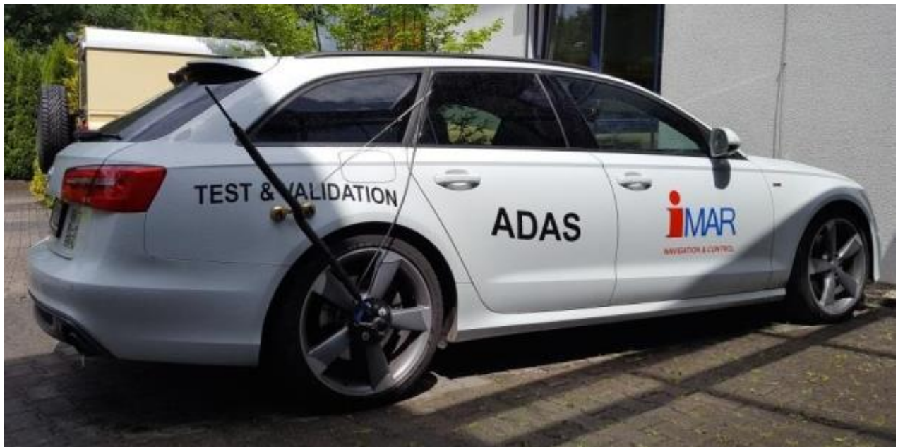
Figure 1: Wheel Sensor to measure vehicle’s speed precisely
