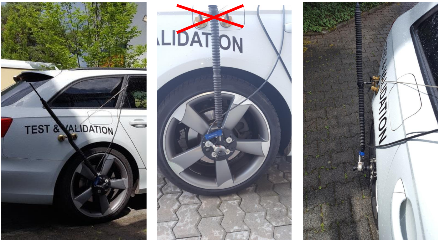
Figure 2: Fix the vacuum cup mountings on rigid surface (not e.g. on the tank cover)
