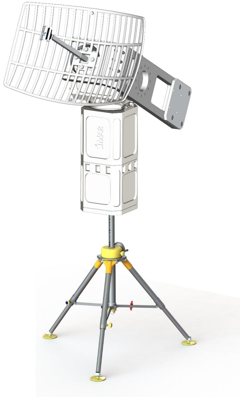
**Figure:** iIPSC-PT-10 for a customer defined grid antenna payload, mounting slot for optional counter weights (depending on the weight of the payload), with heavy duty tripod for quick installation or directly mounted on a vessel, integrated iSCU Stabilization & Control Unit (supporting pointing / tracking using external commands) and optional gyro stabilization
