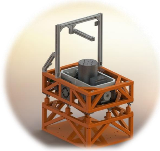
Figure 2: 3-axes Gimbal for Cold Atom Gravimeter Stabilization (example)
