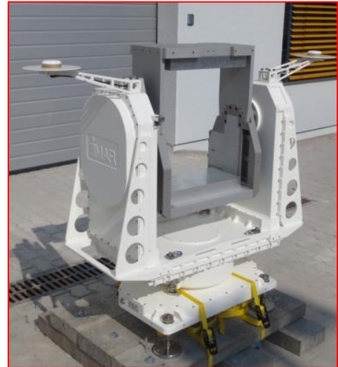
Figure 12: Setup with two GNSS Antennas on Platform iPSC-MSG
