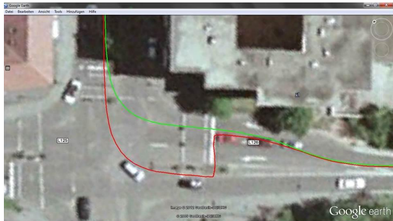
Figure 3: Behavior in urban canyons (9 m distortion of loosely coupled solution against deeply coupled solution)
