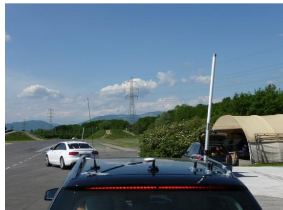
Figure 5: Antenna setup on two test vehicles (GNSS, Radio Modem, WLAN for inter-vehicle-communication)
