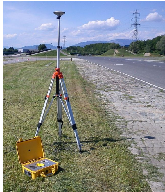
Figure 7: For autonomous users – using your own GNSS reference station
