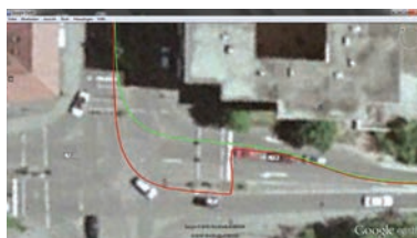
(Figure 1, above) Advantage of deeply coupled architecture (Figure 2, right) Behaviour in urban canyons (9m distortion with loosely coupled solution against deeply coupled solution)
