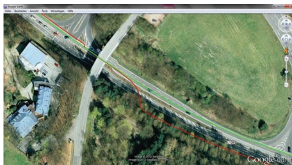
(Figure 1, above) Advantage of deeply coupled architecture (Figure 2, right) Behaviour in urban canyons (9m distortion with loosely coupled solution against deeply coupled solution)
