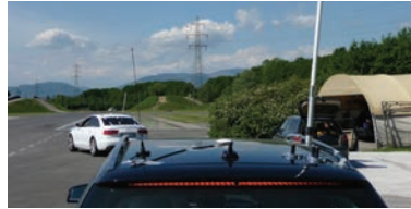
(Figure 3) Antenna setup on two test vehicles (GNSS, radio modem, WLAN for inter-vehicle communication)
