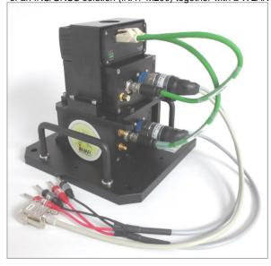
managed router and a LTE / UMTS / GSM modem, all mounted together on a single carrier. This light weight small carrier contains also mounting brackets and grasps for easy handling. As an option, an integrated rechargeable battery can be made available to bridge power interrupts of up to several minutes. The size of the carrier base is approx. 230 mm x 230 mm.
