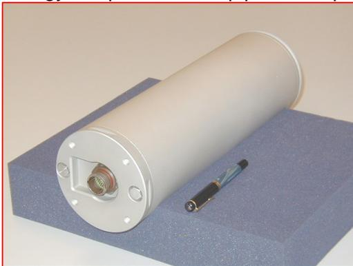
tool in a pipeline can be exactly determined. To achieve this, the inspection tool is coupled with a inertial Pipeline Surveying Tool (iPST) consisting of three gyroscopes, three accelerometers, odometers and an electronic device for signal processing. The gyroscopes are used to determine attitude and heading of the iPST. The accelerometers and the odometers are used to determine the translational motions. All data are processed using a filter which also permits additionally available
