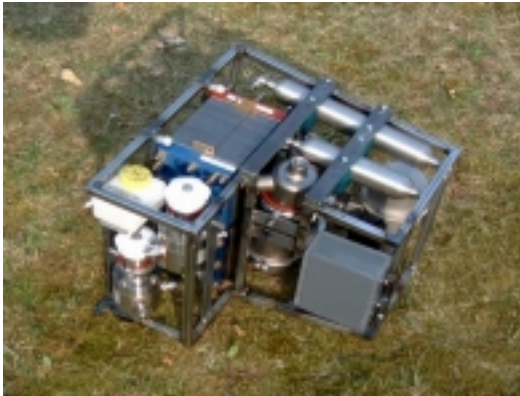
Fig.2.: Fuel Cell System
