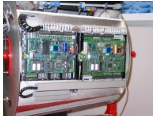
Fig.3.: Power Distribution Electronics
