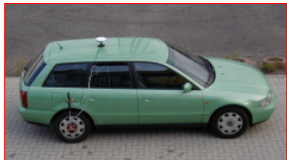
iNAV-FJI-LSURV on a surveying vehicle, equipped with Omnistar DGPS and wheel mounted odometer
